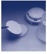
Place membrane onto solid or liquid medium and incubate. Discard the base. (It's also recyclable.)
