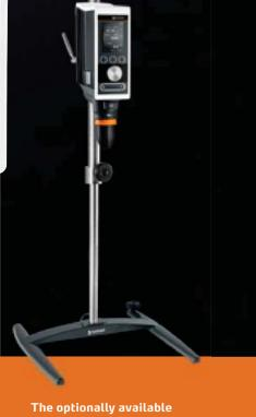
telescope stand almost completely compensates for the weight of the overhead stirrer. Makes it easy to change vessels or tools in no time at all.
