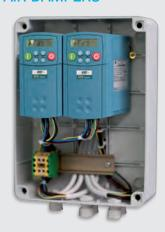
Extracted air flow can be automatically regulated by variable air volume system (VAV), keeping constant air velocity on the frontal sash area. Control is performed by inverter to set fan power, or dampers to modulate air flow ventilation. LOGIKA fume cupboards are **Bureau Veritas certified** for variable air volume (**EN 14175 part 6** european standard).
