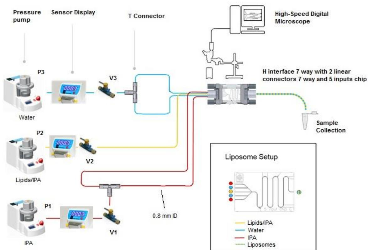
Figure 3. Schematic showing representative setup of a nanoliposome system.
