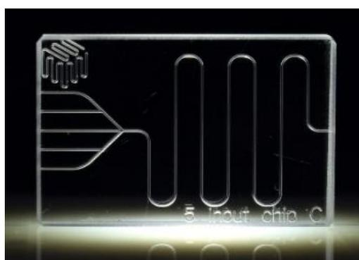
Figure 5. 5 Input Chip - Long Channel.
