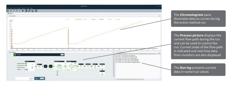
Fig 6. System control module showing Chromatogram pane, Process picture, and Run log features simultaneously.
