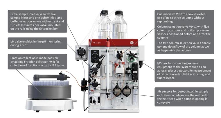
Fig 4. Optional components can be added in the two empty positions in the system chassis or mounted on rails to expand the capability of the ÄKTA go system. A total of maximum six options can be added at the same time.
