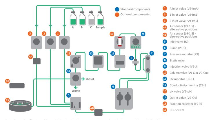
Fig 2. Flow path of ÄKTA go with standard and optional components that may be added to expand the capability of the system.
