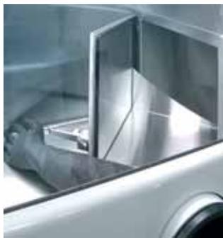
The Biowizard BW-3 is a Class III safety cabinet which protects the operator and the environment from hazards in handling infected and other dangerous biological material.
