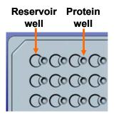
**Figure 2.** Each Crystal*EX* crystallization microplate has 96-round buffer reservoir wells and 96 conical flat bottom protein wells.
