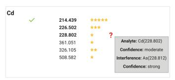
IntelliQuant Star ranking output for Cd. A five-star ranking with green check mark indicates Cd 214 wavelength to be the best. The red question mark indicates there is an issue on Cd 228, and the pop-up tip indicates the Cd 228 result has only moderate confidence as it has a strong arsenic interference.
