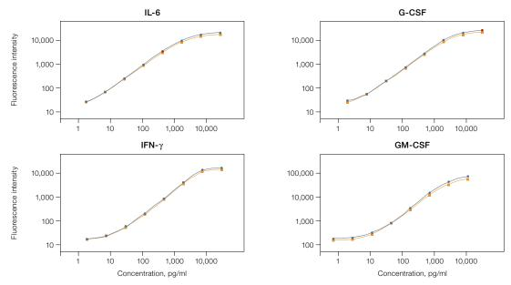
Fig. 2. Standard curve comparison when the Bio-Plex Pro human cytokine 27-plex panel is run on the laser-based Bio-Plex 200 system (
