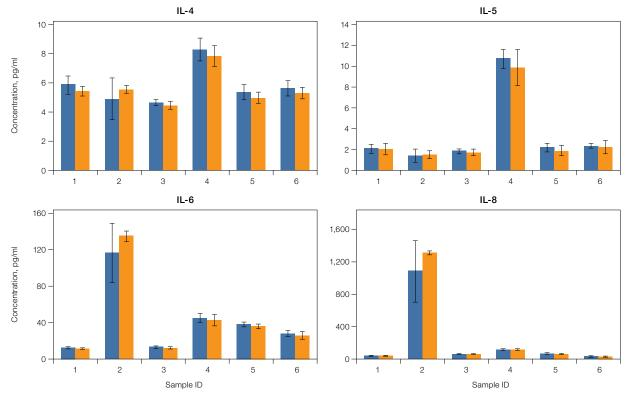
Fig. 3. Sample concentrations obtained using the Bio-Plex 200 (■) and Bio-Plex MAGPIX systems (■).
