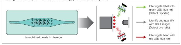
$Fig.\ 1.\ Comparison\ of\ a\ traditional\ flow\ cytometry-based\ system\ with\ an\ LED/image-based\ system.$
