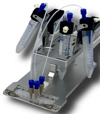
PreciGenome's droplet generation package is also available with an iFlow Light pressure controller. This setup is more affordable and compact. External pressure source and display unit are required for full functionality.
