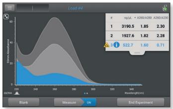
View multiple samples at once on your measurement screen. Here Acclaro has flagged dsDNA sample #3 for the presence of a contaminant.
