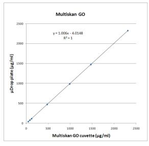
Figure 4. Correlation of the Multiskan GO  $\mu Drop$  Plate low-volume area to the Multiskan GO cuvette measurements
