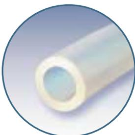
**Sta-Pure** has a unique composite construction of silicone in a PTFE lattice giving it superior burst resistance up to 7 bar (100psi) and 18 times longer life than silicone tubing. It produces virtually no spalling, is USP Class VI approved and is classified as non toxic. Working temperature range 0C to 80C. Opaque white. Autoclavable, SIP and CIP compatible.
