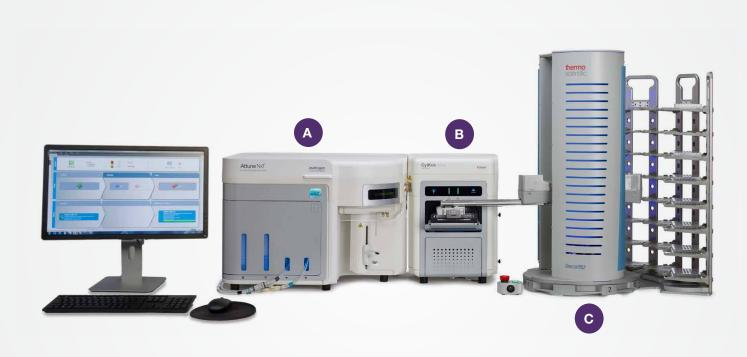
Figure 2. The Attune NxT Flow Cytometer configured for robotic automation with the Orbitor RS2 Microplate Mover. The components include the (A) Attune NxT Flow Cytometer, (B) CytKick Autosampler, and (C) Orbitor RS2 Microplate Mover.
