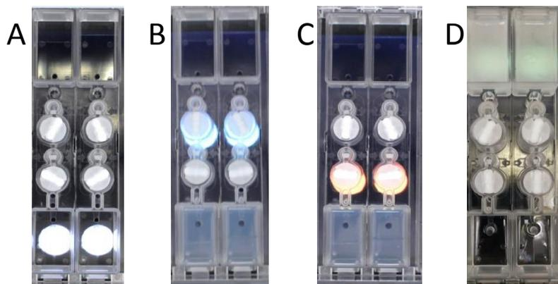
Guide lights underneath the Nadia cartridge chips indicate loading positions for the emulsion oil (A), beads (B) and cells (C), and direct the user to the emulsion (D) after the run is complete.
