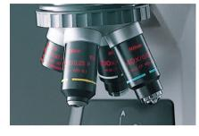
distances and higher N.A.'s to deliver startlingly clear images at any magnification because chromatic aberrations are corrected over the entire field of view. Nikon CFI optics employ an eco-glass that is manufactured with no harmful substances such as lead and arsenic.
