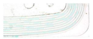
A portion of the storage coil with picoliter droplets. Individual droplets are not easily visible, however clusters can be seen. Each of the droplets in the cluster is about 100 µm in diameter.
