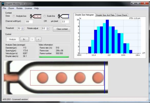
Screenshot of Droplet monitor software. An imported video file is analyzed to give the droplet size and drpolet production rate variation over the duration of the video.
