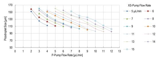
Size dependence on flow rate. XS-Pump flow rate Q<sup>-</sup> range shown in legend.
