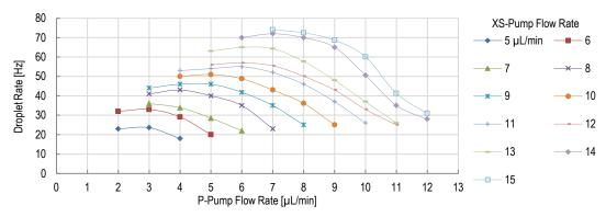
Droplet breakup rate dependence on flow rate. XS-Pump flow rate Q- range shown in legend.
