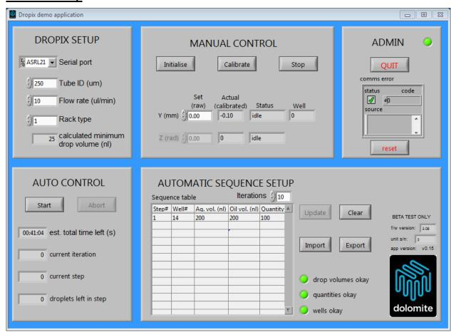
Screenshot of Dropix Software setup. Well # 14 of the Sample strip is loaded with dilute food coloring. The Flow Rate option is the DROPIX SETUP section of the software is updated manually to match the flow rate set on the XS-Pump.
