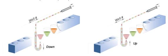
Droplet on demand – a constant suction driven flow results in the creation of a segmented flow. The timing of the 'up' or 'down' position of the sampling hook dictates the droplet volume and spacing volume respectively. The transverse position of the hook dictates the selection of the sampling well.
