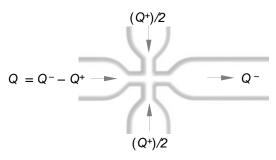
Detailed view of the flow focussing junction illustrating the flow distribution. (Net flow rate at Dropix) = (Suction from Syringe pump) – (Infusion rate of P-Pump)
