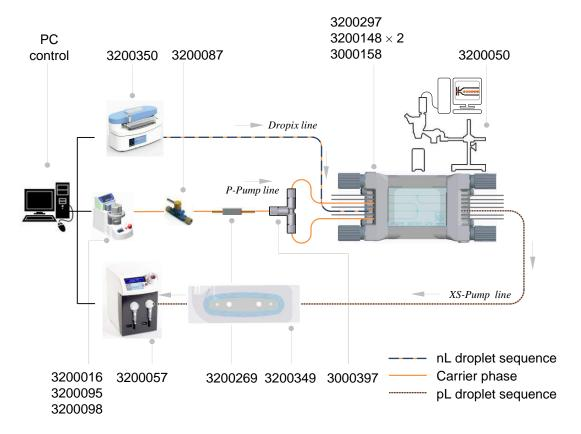
Setup schematic. Yellow lines represent fluorocarbon carrier with 0.1 % surfactant, blue/yellow segmented lines represent nanoliter plugs made from Dropix. PC control is achieved via 'Flow Control Center' software. Image not to scale.
