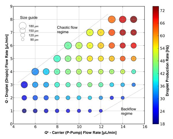
Phase Diagram: Droplet size and production rate dependence on flow rates.
