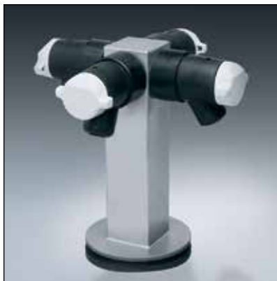
7522200 4-Port Manifold 9.0" h x 8.7" w x 8.7" d (22.9 cm x 22.1 cm x 22.1 cm). Type 304 stainless steel, complete with four neoprene valves with molded plastic knobs that accommodate both 1/2" and 3/4" adapters for connection of flasks. Shipping weight 2 lbs. (1 kg) 1, 2.5, 4.5A, 4.5P
