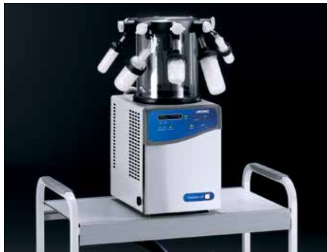
FreeZone 2.5 Liter Benchtop Freeze Dry System 7670520, Clear Chamber with Valves 7443500, Portable Table 8025000 and miscellaneous glassware.
