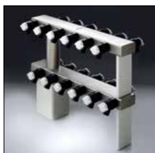
7548000 24-Port Two-Tier Manifold 20.0" h x 26.4" w x 10.6" d (50.8 cm x 67.1 cm x 26.9 cm), type 304 stainless steel, complete with 24 neoprene valves with molded plastic knobs that accommodate both 1/2" and 3/4" adapters for connection of flasks. Shipping weight 20 lbs. (9 kg) 6, 12, 18
