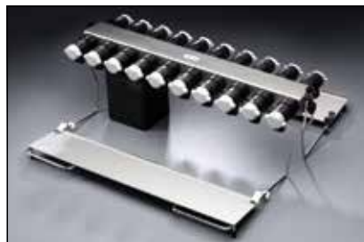
7522500 20-Port Manifold with Support Shelves 10.0" h x 29.6" w x 24.2" d (25.4 cm x 75.2 cm x 61.5 cm). Type 304 stainless steel, complete with twenty neoprene valves with molded plastic knobs that accommodate both 1/2" and 3/4" adapters and two adjustable aluminum support shelves with stainless steel rods. Shipping weight 15 lbs. (7 kg) 6, 12, 18
