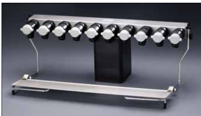
7522400 10-Port Manifold with Support Shelf 10.0" h x 29.6" w x 14.6" d (25.4 cm x 75.2 cm x 37.1 cm). Type 304 stainless steel, complete with ten neoprene valves with molded plastic knobs that accommodate both 1/2" and 3/4" adapters and adjustable aluminum support shelf with stainless steel rods. Shipping weight 11 lbs. (5 kg) 6, 12, 18
